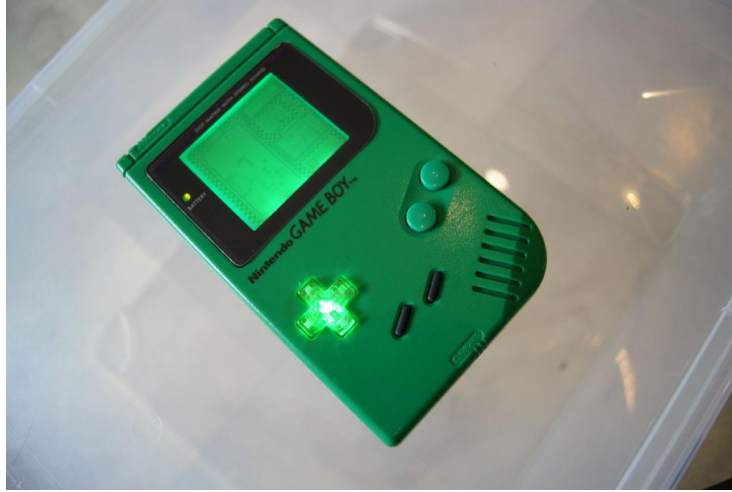
Figure 73. An example of using an LED behind the D-pad (plus sign buttons on the left), as well as customized case, buttons, and a backlight mod. Source: chipmusic.org/forums/topic/7345/customized-gear-thread/page/14/
