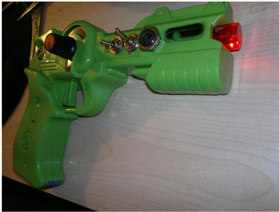
Figure 27. Adding a potentiometer (knob) to control the pitch, toggle switches to pitch down or loop, and a ¼” audio jack to a toy gun. Source:
