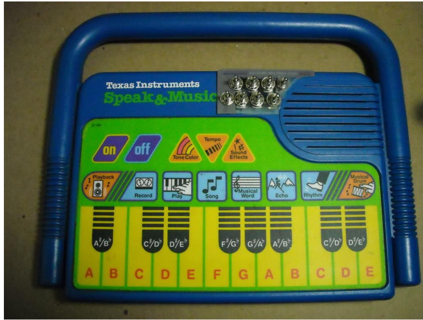
Figure 91. Adding switches to a “Speak & Music” toy. Source: chipmusic.org/forums/topic/4136/bent-circuits-by-greightbit/
