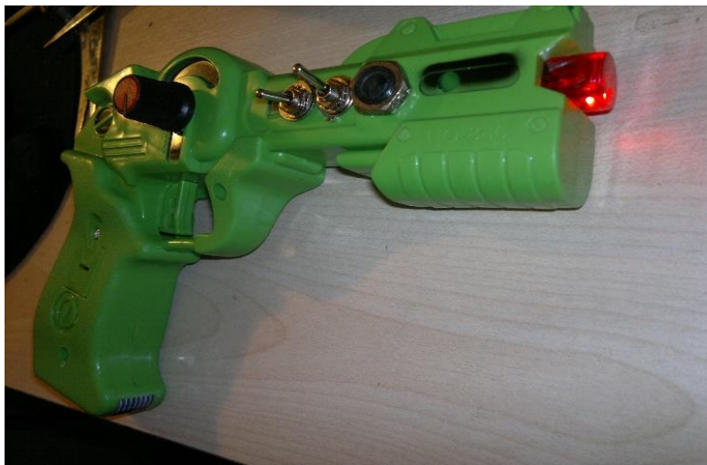
Figure 94. Adding a potentiometer (knob) to control the pitch, toggle switches to pitch down or loop, and a 1/4" audio jack to a toy gun. Source: chipmusic.org/forums/topic/14499/circuit-bent-stylophone-beatbox-circuit-bent-toy-gun/
