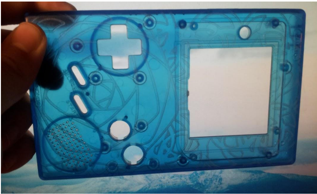
Figure 66. Laser engraving a DMG case. Source: chipmusic.org/forums/topic/12223/laser-engraving-take-two/page/4/
