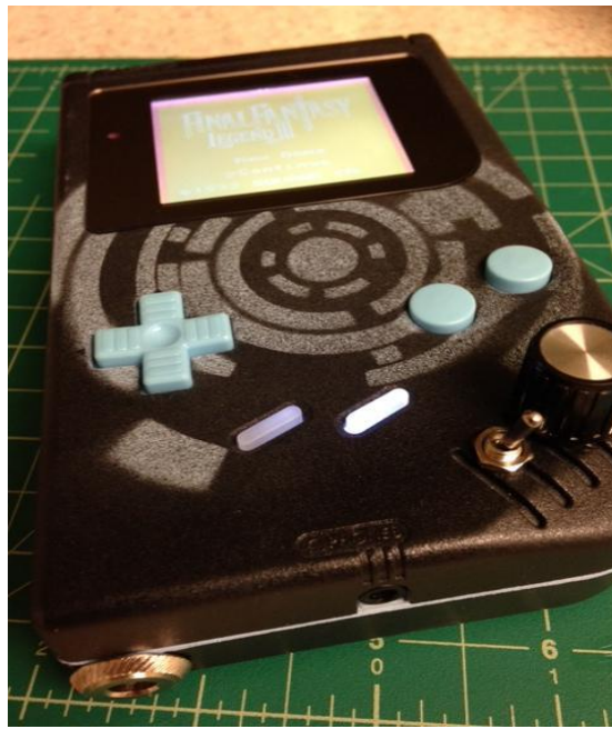
Figure 23. A DMG with artwork (aesthetic mod), LEDs behind the start and select buttons (the two buttons in the center near the bottom), prosound audio mod (audio jack on the bottom left), and a clock mod (also known as a “pitch mod”) with switch and potentiometer (on the bottom right). Source:
