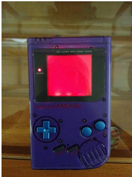
Figure 86. An example of an inverted red backlight installed in a DMG. Source: chipmusic.org/forums/topic/7345/customized-gear-thread/page/2/
