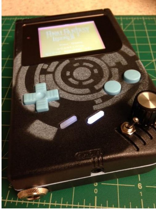
Figure 89. A DMG with artwork, LEDs behind the start and select buttons, prosound audio mod, and a clock mod with switch and potentiometer (also known as a “pitch mod”). Source: chipmusic.org/forums/topic/7345/customized-gear-thread/page/59/
