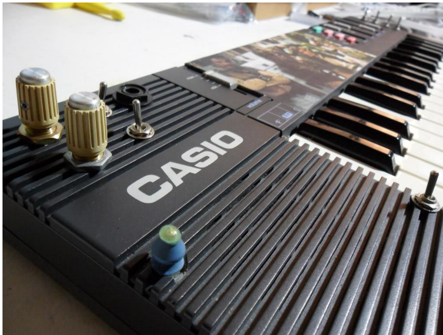
Figure 92. Adding switches and potentiometers (knobs) to a Casio Synthesizer. Source: chipmusic.org/forums/topic/4136/bent-circuits-by-greightbit/
