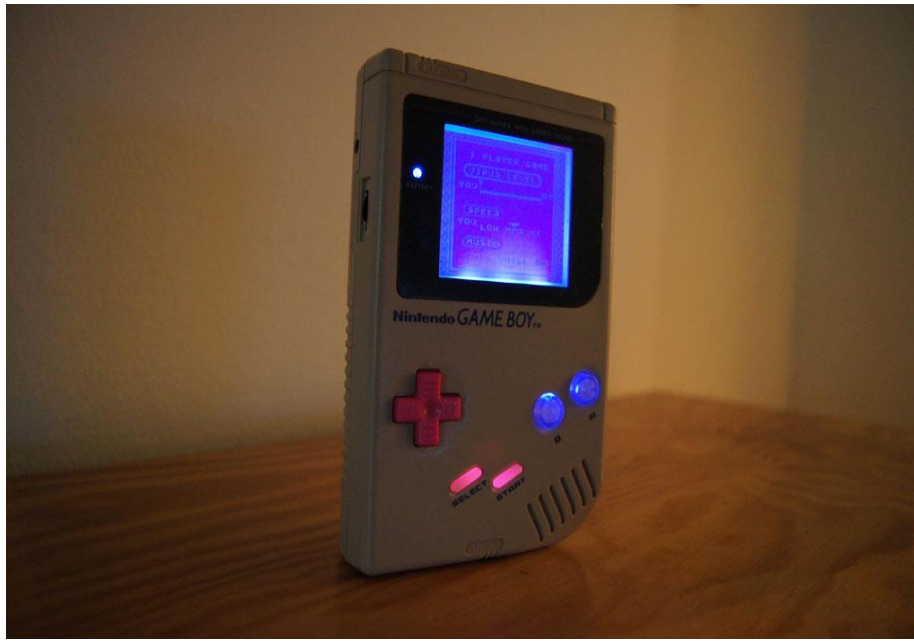
Figure 87. An example of a backlight mod with backlit buttons. Source: chipmusic.org/forums/topic/7345/customized-gear-thread/page/14/
