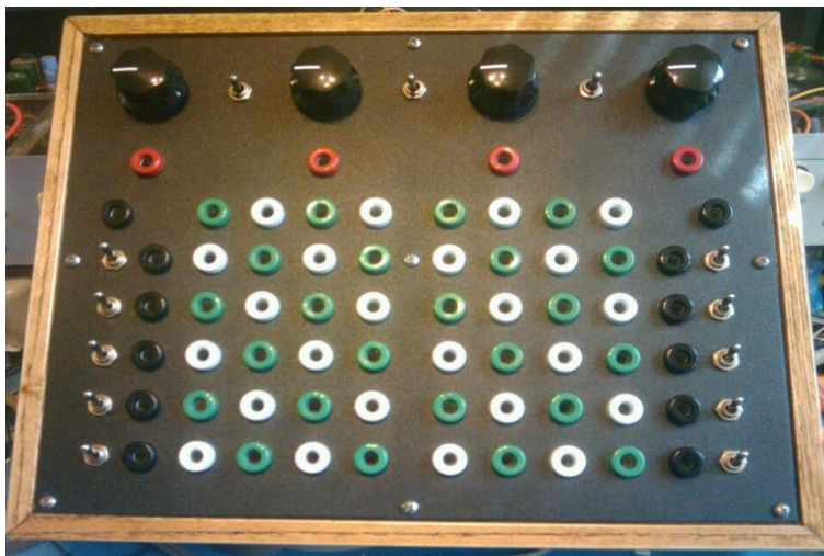
Figure 28. An image of a “Universal Bend box,” which enables experimentation with connecting or altering up to 24 bend points on a circuit-bendable device using a common serial connector (DB25). Source: chipmusic.org/forums/topic/1121/universal-bend-box/
