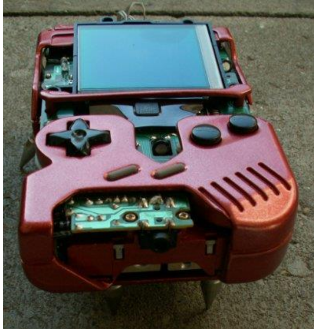
Figure 79. Modifying a DMG by removing pieces to expose the electronics. Source: chipmusic.org/forums/topic/7345/customized-gear-thread/page/12/
