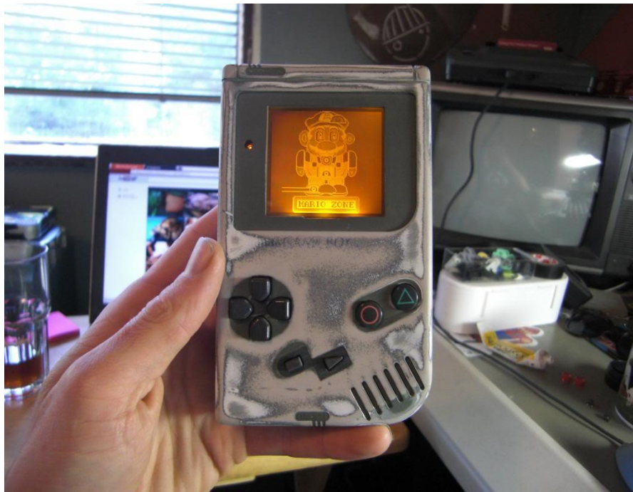
Figure 78. Replacing DMG buttons with buttons from a Playstation controller, custom backlight mod, and custom case design. Source: chipmusic.org/forums/topic/10130/d3th-st4r-wild-builds-nonsense/page/9/
