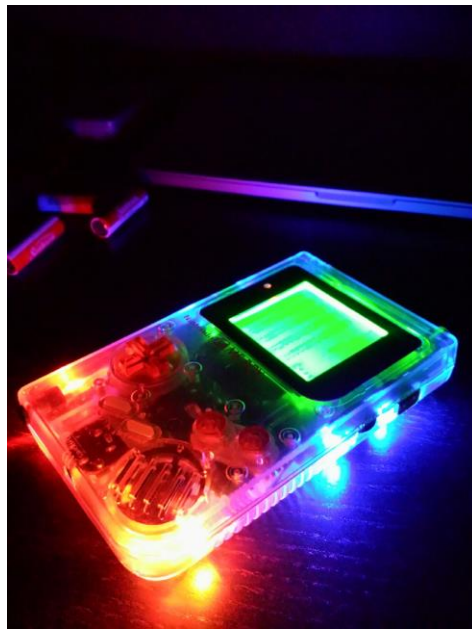
Figure 70. An example of a multicolored LED and a backlight mod. Source:
