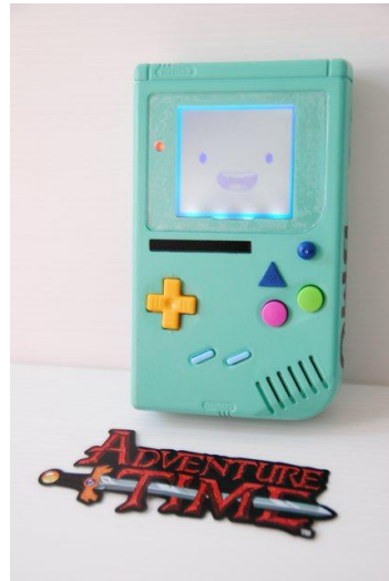
Figure 77. Modifying a DMG's case, buttons, and backlight to resemble a character from a television show. Source: chipmusic.org/forums/topic/7345/customized-gear-thread/page/72/
