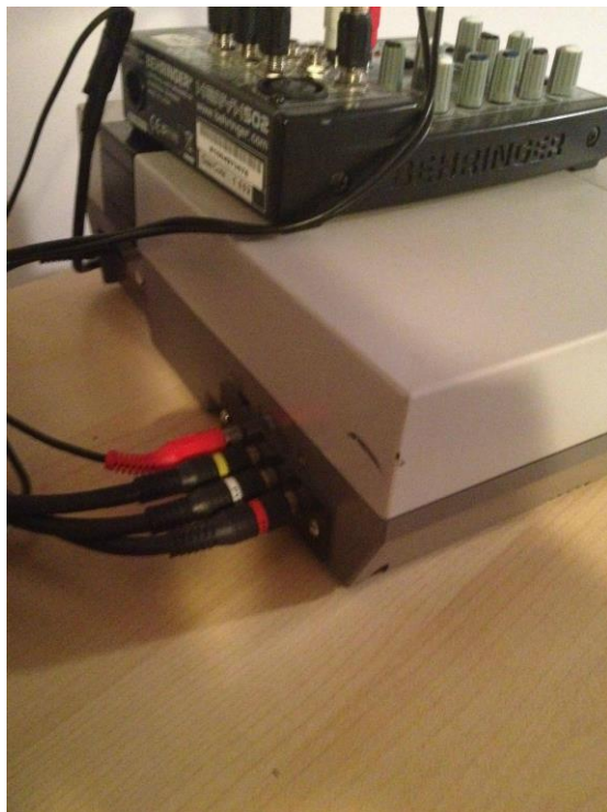
Figure 83. Adding one video and three audio outputs to the Nintendo Entertainment System (NES). Source: chipmusic.org/forums/topic/7345/customized-gear-thread/page/17/
