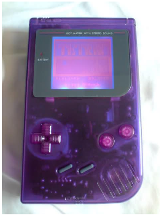
Figure 85. An example of an inverted pink backlight installed in a DMG. Source: chipmusic.org/forums/topic/7345/customized-gear-thread/page/8/
