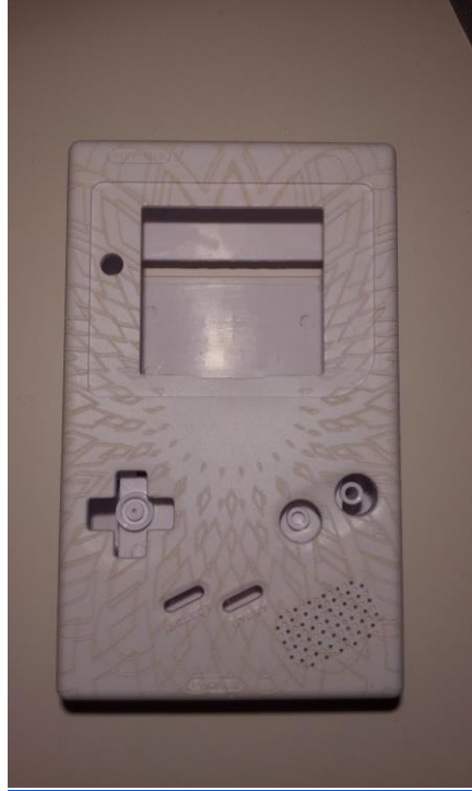
Figure 69. Laser engraving a DMG case. Source:
