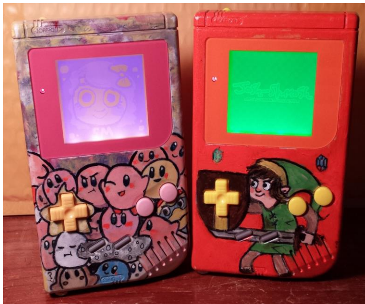
Figure 60. An example of customizing a DMG case as well as two different backlight mods. Source: chipmusic.org/forums/topic/7345/customized-gear-thread/page/61/
