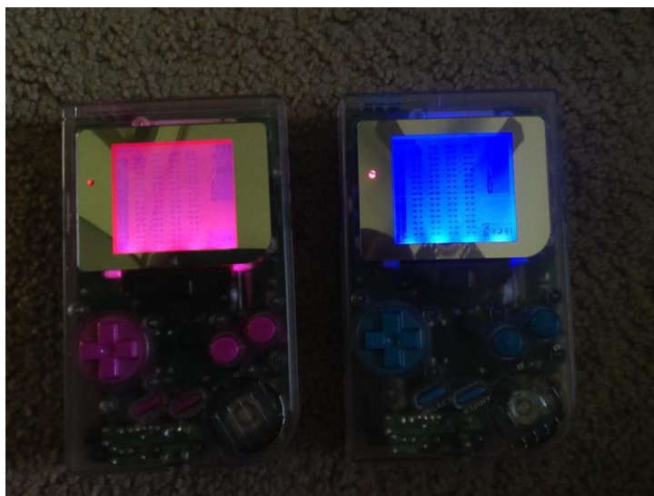
Figure 84. Two DMGs with backlight mods. Source: chipmusic.org/forums/topic/7345/customized-gear-thread/page/70/288
