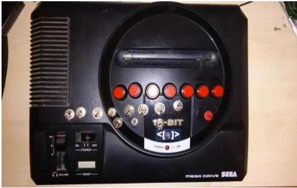
Figure 95. Adding several buttons and switches for both audio and video bends on a Sega Mega Drive. Source: chipmusic.org/forums/topic/14965/circuit-bent-megadrive-lotus-ii-rewire/
